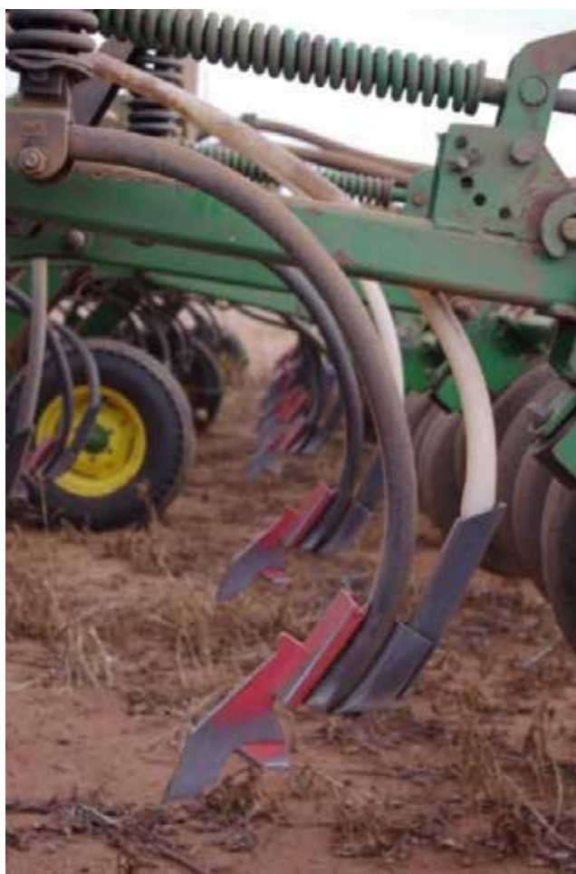
Photo: Typical knife point and press wheel setup that is ideal for incorporating Valor prior to sowing winter crops.
